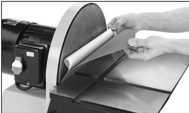
Figure 31. Example photo of installing the sandpaper disc.
